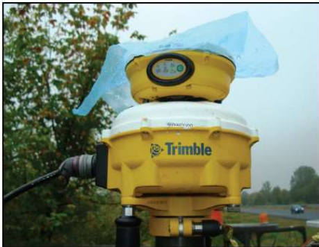
Figure 14. Validation of roller mounted GPS with a hand-held rover.
