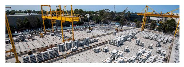
Need to model precast segment supply against Tunnel Boring Machine (TBM) demand.
