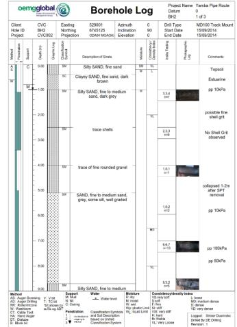
Boreholes result in a highly disturbed, non-continuous and highly interpreted understanding of the ground.
