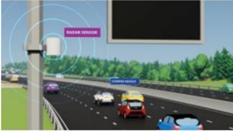
Stopped Vehicle Detection Retrofit
