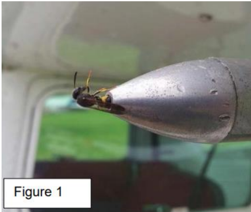
Figure 1. Mud dauber wasp emerging from an uncovered pitot tube. (Source:backcountrypilot.org)
